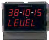
PD2-6001 Helios Feet & Inches Level Meter Input: 0-20 mA, 4-20 mA; ±10 VDC (0-5, 1-5, 0-10 V)
