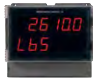
PD2-6100 Helios Strain Gauge Meter Input: 15, 30, 150, 300 mV unipolar; ±15, ±25, ±150, ±250 mV bipolar
