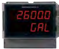
PD2-6000 Helios Process Meter Input: 0-20 mA, 4-20 mA; ±10 VDC (0-5, 1-5, 0-10 V)
