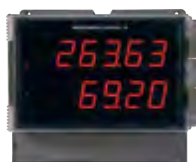
PD2-6363 Helios Dual Pulse Input Flow Rate/Totalizer Input: Dual pulse, open collector, NPN, PNP, TTL, switch contact, sine wave (coil), square wave
