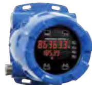
PD8-6363 ProtEX-MAX Explosion-Proof Pulse Dual-Input Flow Rate/Totalizer Input: Dual Pulse, open collector, NPN, PNP, TTL, switch contact, sine wave (coil), square wave
