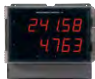
PD2-6400 Helios High Voltage & Current Meter Input: High Voltage: (Channel V) 0-300 VDC or VAC; High Current: (Channel A) 0-5 AAC or ADC. Modbus PV (Slave)
