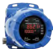
PD8-6210 ProtEX-MAX Explosion-Proof Analog Input Batch Controller Input: 0-20 mA, 4-20 mA; ±10 VDC (0-5, 1-5, 0-10 V)
