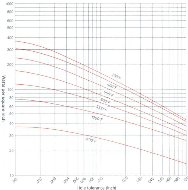
**Figure 3:** Maximum watt density for Superwatt swaged cartridge heaters with various increasing temperatures and hole tolerances. Source: Backer Hotwatt
