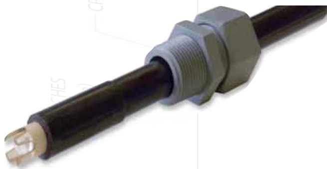
The P585 Combination probe is a combination glass electrode encapsulated in 3/4" epoxy body and comes with a 3/4" NPT compression fitting.
