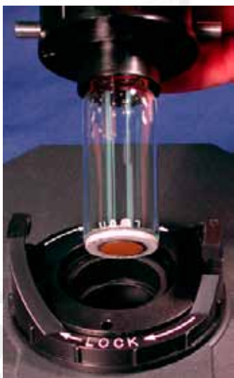
The ultrasonic cleaning system insures that the optical chamber is clean whether clean or raw water is being measured.
