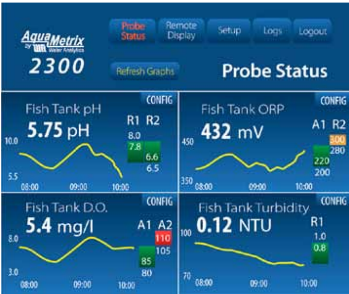
The web display shows as many panes as there are sensors—in this case four. Each pane shows the process value, time trace, relay settings, alarm settings and status. Configuring and calibrating each sensor is a click away.
